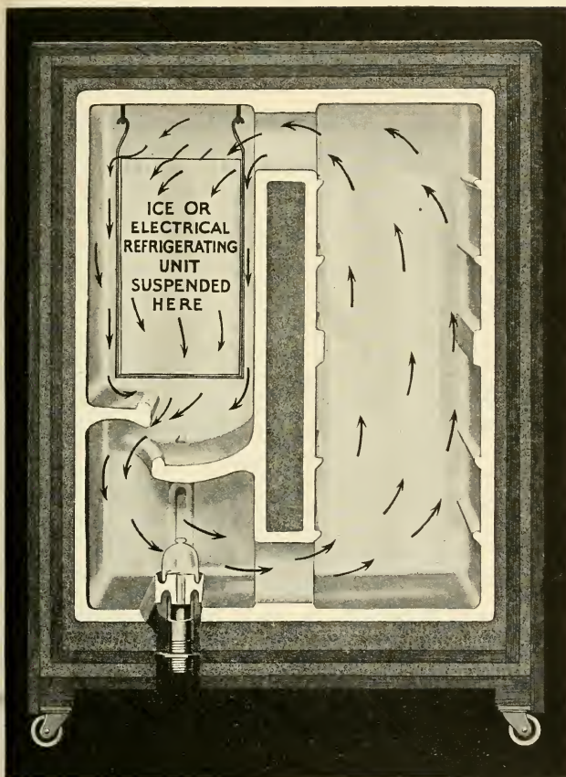
FIG. 173.—SECTION OF JEWETT SOLID PORCELAIN REFRIGERATOR SHOWING CORK INSULATION.
