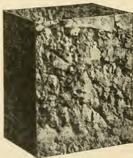
FIG. 208.—PURE CORKBOARD INSULATION USED BY MECHANICOLD.
